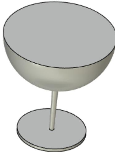
After selecting the removed face, the shell will be built for the entire body, and not just for its spherical part.
